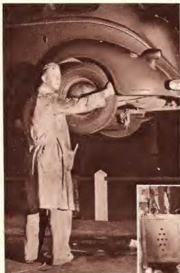
When your car is on a hoist, test the wheels for dragging brakes. You can do this at home by jacking up the wheels.
